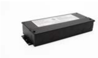
TLD24V-192W 192W Class 2 LED driver 100-277V input, 24V output x2 (2x 96W output) TRIAC, ELV, MLV, Forward & reverse phase, PWM output 1/2" knockout size Wet locations rated Dimensions: 10.9" x 4.3" x 1.8" (278mm x 110mm x 40mm)
