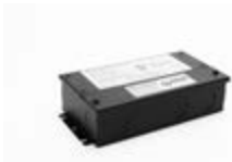
TLD24V-30W 30W Class 2 LED driver 100-277V input, 24V output TRIAC, ELV, MLV, Forward & reverse phase, PWM output 1/2" knockout size Wet locations rated Dimensions: 6.5" x 3.7" x 1.6" (165mm x 94.5mm x 40mm)
