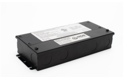
TLD24V-96W 96W Class 2 LED driver 100-277V input, 24V output TRIAC, ELV, MLV, Forward & reverse phase, PWM output 1/2" knockout size Wet locations rated Dimensions: 8.7" x 3.7" x 1.6" (220mm x 94.5mm x 40mm)
