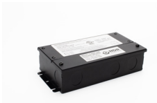
TLD24V-30W 30W Class 2 LED driver 100-277V input, 24V output TRIAC, ELV, MLV, Forward & reverse phase, PWM output 1/2" knockout size Wet locations rated Dimensions: 6.5" x 3.7" x 1.6" (165mm x 94.5mm x 40mm)
