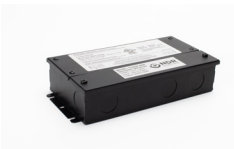
TLD24V-60W 60W Class 2 LED driver 100-277V input, 24V output TRIAC, ELV, MLV, Forward & reverse phase, PWM output 1/2" knockout size Wet locations rated Dimensions: 7.4" x 3.7" x 1.6" (188mm x 94.5mm x 40mm)
