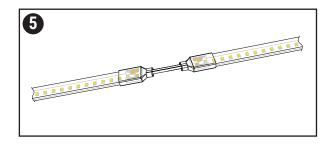
When using tape to tape joiner connector, follow the step by step guide above for both connections.
