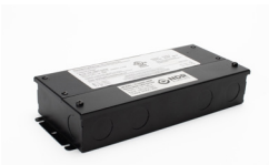
TLD24V-96W 96W Class 2 LED driver 100-277V input, 24V output TRIAC, ELV, MLV, Forward & reverse phase, PWM output 1/2" knockout size Wet locations rated Dimensions: 8.7" x 3.7" x 1.6" (220mm x 94.5mm x 40mm)
